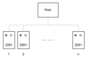
Install the OMNIKEY 2061 Bluetooth reader with no more than eight hosts. Installing the reader on a ninth host, removes the first reader instance from the host reader list.
