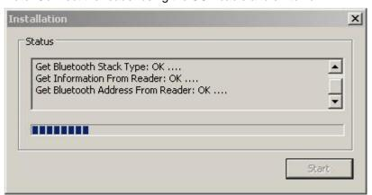
Clicking **Start** pairs the reader and installs the Bluetooth device driver. After finishing the installation process the reader is ready to use.
