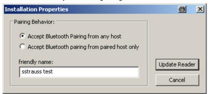
The default option, **Accept Bluetooth Pairing from any host** indicates that the reader accepts pairing requests from computers which are currently not paired with the reader.
