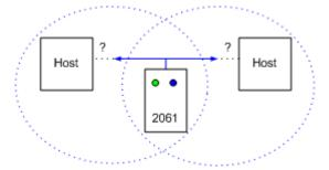
When an OMNIKEY 2061 Bluetooth reader is installed on more than one host and the Bluetooth field of this host overlaps, it is unpredictable to which of the hosts the device will connect. Overcome this issue by using Bluetooth radios with reduced transmission power. For instance the Bluetooth Class 3 radio (max. range 1m) has reduced transmission power so that the Bluetooth field area does not overlap.
