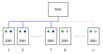
When more than seven readers are installed on one host, if these readers are enabled and in range of the hosts Bluetooth radio, it is unpredictable which readers are connected.
